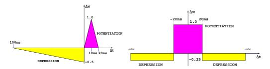
Fig. 2. Asymmetrical STDP temporal window for excitatory (left) and symmetrical STDP temporal window for inhibitory (right) synapse adaptation (from [29]).
