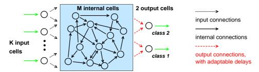
Fig. 1. Architecture of the spiking neuron network. The reservoir is the internal network (the colored square) and green (light grey) links represent the interface with environment. The network is presented for C=2 classes.
