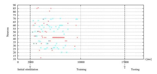
Fig. 14. The 80 excitatory neurons of the reservoir have been marked by a red (black) "+" for class 1 or a blue (light grey) "x" for class 2 each time they play the role of pre-synaptic neuron of a triggering connection producing a readout delay change.
