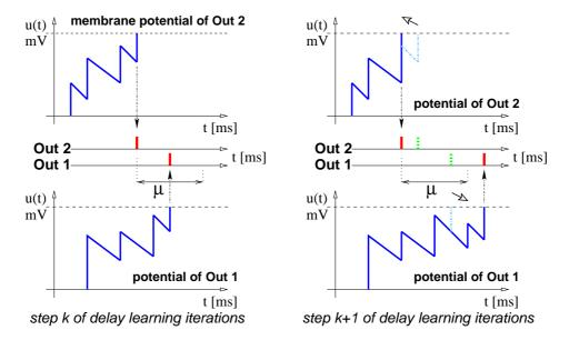
Fig. 3. An example illustrating the effect of one iteration of the delay learning algorithm on the firing times of the two readout neurons.
