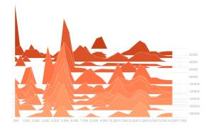
Figure 5. Histogram of discrete latent usage for sliced DVQ with  $n_d=2$  and  $\log_2 K=14$ . The x-axis corresponds to the different possible discrete latents, while the y-axis corresponds to the progression of training steps (time increases in a downwards direction). Notice the diversity of latents used in this case.
