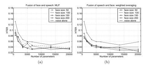
**Fig. 3.** (a) HTER for MLP fusion vs. number of Gaussians and face template size. (b) HTER for weighted averaging fusion vs. number of Gaussians and face template size.
